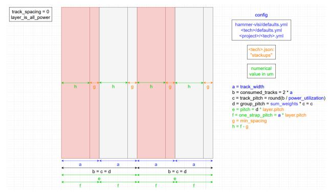
For track spacing = 0 and effective power utilization < 100%, powerstraps are routed as follows.
