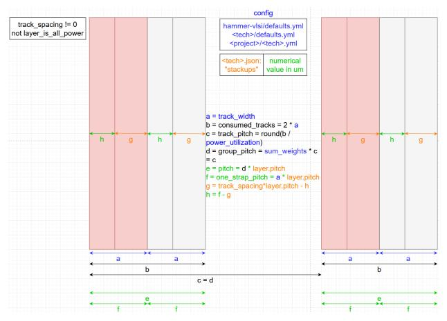
The currently supported API supports power strap generation by tracks, which auto-calculates power strap width, spacing, set-to-set distance, and offsets based on basic DRC rules specified in the technology Stackup object. The basic pieces of information needed are the desired track utilization per strap and overall power strap density. Different values can be specified on a layer-by-layer basis by appending \_<layer name> to the end of the desired option.
