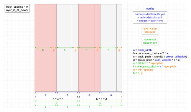
For track spacing = 0 and effective power utilization < 100%, powerstraps are routed as follows.
